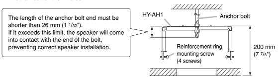
**Step 3.** Mount the ceiling reinforcement ring (supplied with the speaker) to the Hanging Bracket.
